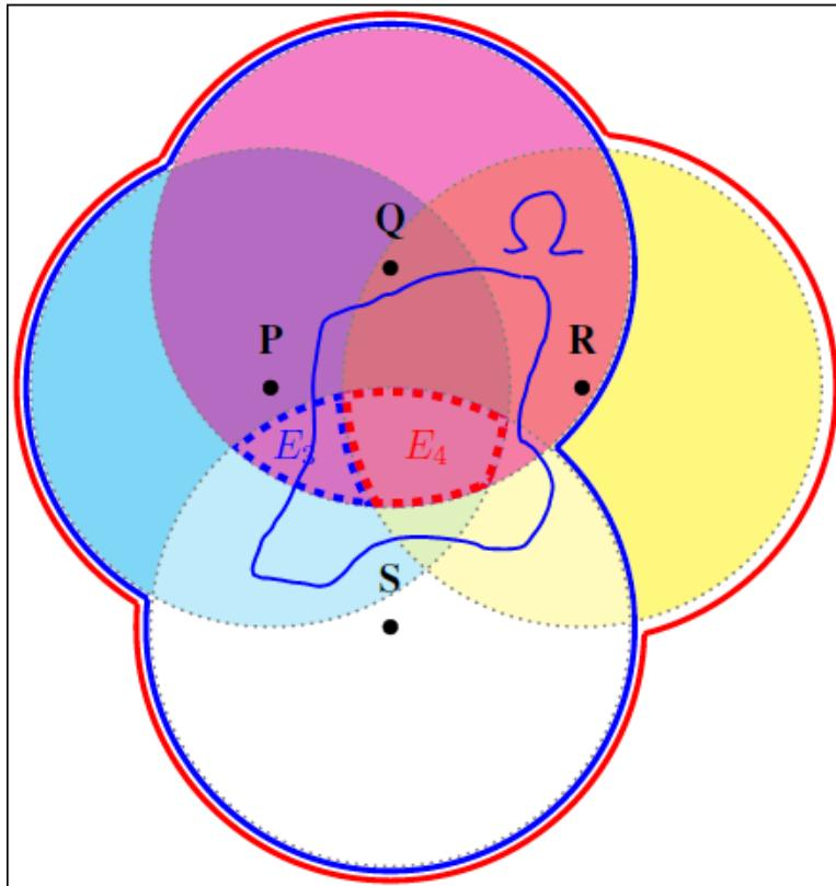
Rate of successful transmissions  $S_L(\Omega)$  from end devices on any compact subset  $\Omega$  of the plane to at least  $L$  gateways among the ones reachable by each end device  $\in \Omega$
